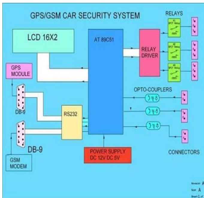
**Fig. 2.5 Block diagram**
