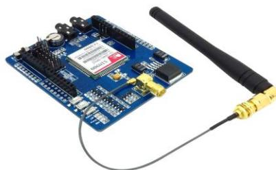
**Fig 2.4 GSM Modem**
