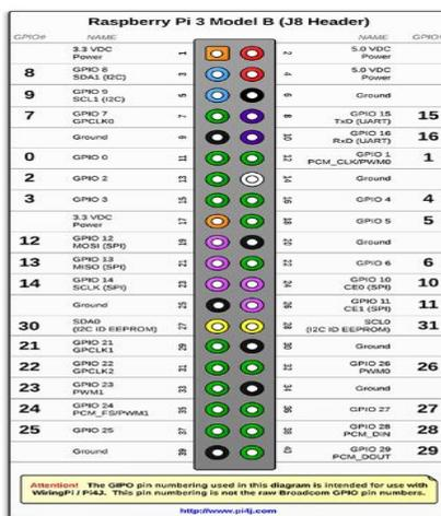
Fig1: Pin diagram of Raspberry Pi
