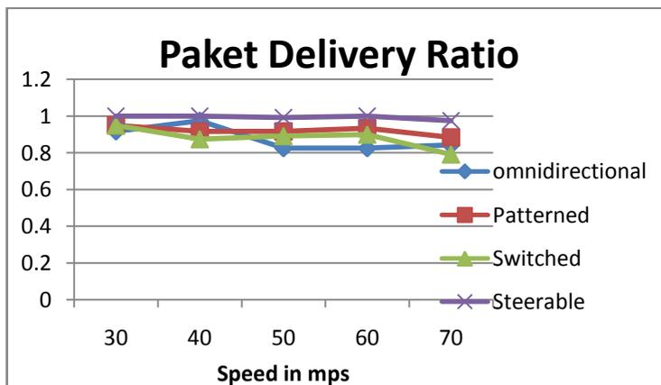
As the speed of flying air vehicle increases pdr for steerable antenna is better than from other antenna. As speed increases pdr for FANET decreases for different antenna.
