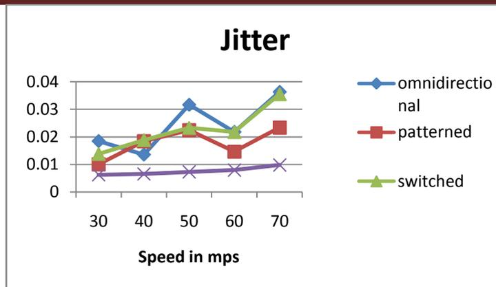
As the speed of flying nodes increases jitter for different antenna increases but steerable antenna jitter is better than other antenna's.
