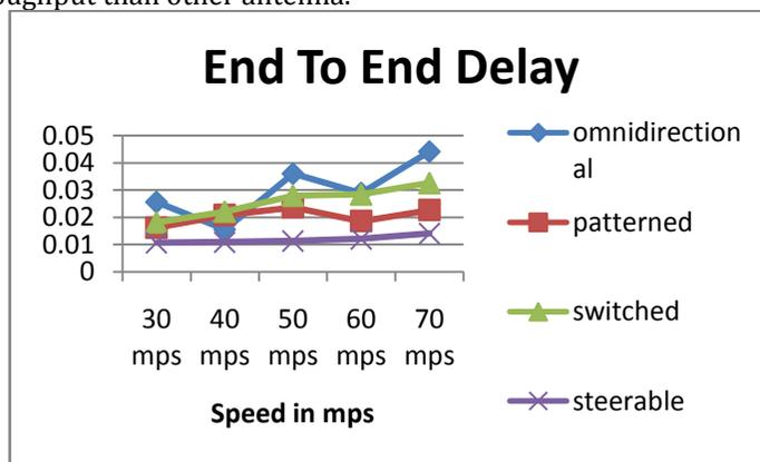
As the speed of air vehicle nodes increases from 30 to 40 mps end to end delay for omni-directional antenna decreases then it increase for high speed of nodes. For switched and patterned antenna as the speed increases end to end delay increases. For steerable antenna end to end delay is minimum from other antenna.
