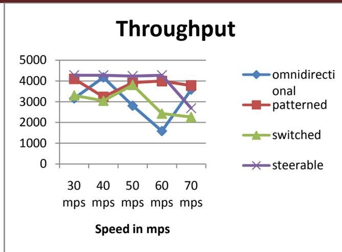
As the speed of flying nodes increases throughput for different antenna's decreases but steerable antenna has better throughput than other antenna.
