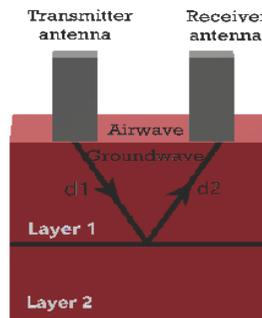
Fig. 2 Ground Penetrating radar
