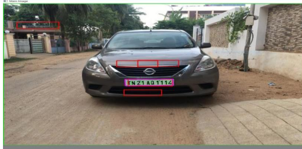
Fig 12: Output on performing character segmentation
