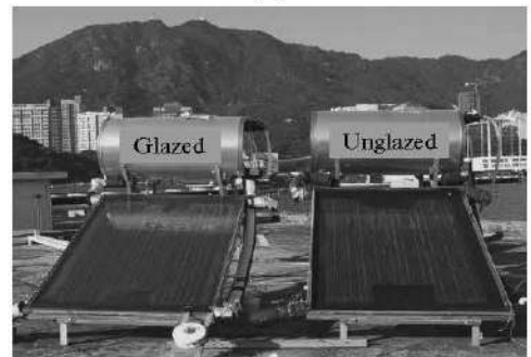
Fig. 4 (a) C/S view of PV-T collector with flat box absorber and multi water design (b) PV-T Collectors with and without glass cover
