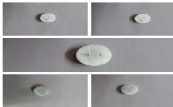
Fig 5 Hardness test specimens after testing
