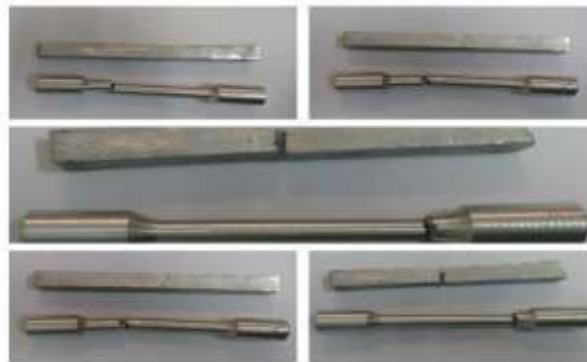
Fig 3 Tensile and bending test specimens after testing
