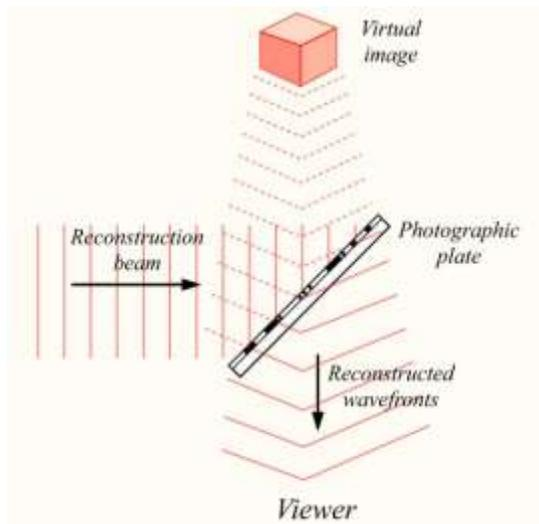
[Fig.1] Reconstructing a hologram
